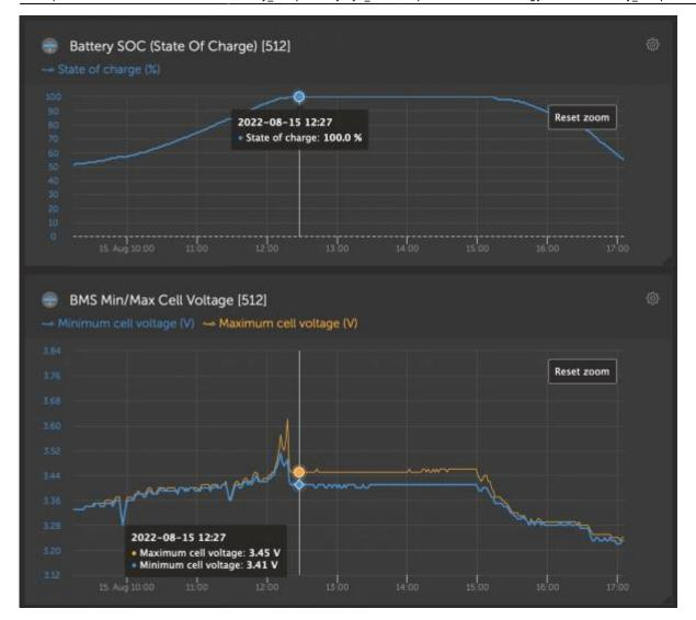
In an imbalanced battery installation, you can see the minimum cell voltage does not rise as much (if at all), compared to the maximum cell voltage. Once the battery is at 100%, the maximum cell voltage does not fall back closely in line with the minimum cell voltage. Any power spikes are disproportionately affecting the high voltage cells, generating alarms, and putting the system at risk of shutting the battery down.
