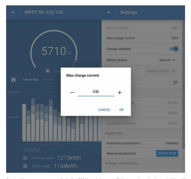
Start with a severe current limit (i.e 50%) and then see if that resolves the issue (while still making
