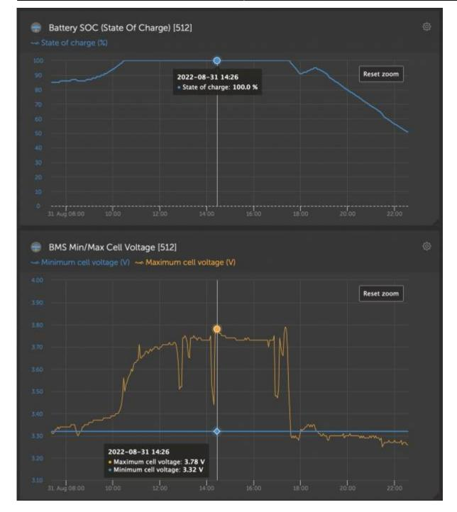
To help the batteries balance quickly, keep the batteries fully charged and the system voltage stable until the errors go away. In an ESS system, set it to 'keep batteries charged', in an off-grid system the fastest way is to either charge / balance the battery before installation, or to fully charge with a generator if not enough solar is available to keep the batteries fully charged.
