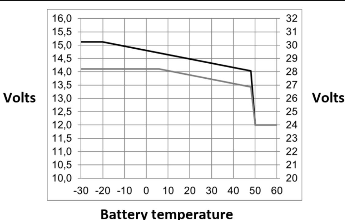
**EN** Default output voltages for Float and Absorption are at 25°C.
